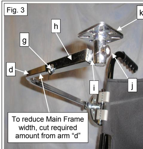
using a hacksaw, finally clearing any swarf before re-installing into Rotation Mount. \*
