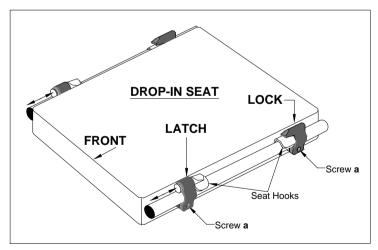
**NOTE:** To enable the Seat Hook Brackets to sit snugly over the Seat Rails, it may be necessary to slacken the M6 Bracket screws to reposition the Brackets as required. Re-tighten screws sufficient to prevent any movement.
